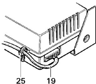
5. For strain relief, secure control panel cable (19) on the control electronics by means of enclosed cleat (25).
